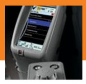
Multi-language LCD monitor and rotary dial provide easy access to machine info and functions. Turn and tap to select work modes, monitor maintenance intervals, check diagnostic codes and set cab temperature. Control oil flow and toggle between dig and thumb modes with a programmable thumb attachment mode.
