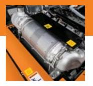
Our FT4 field-proven technology is simple and efficient, employing cooled exhaust gas recirculation (EGR), a diesel oxidation catalyst (DOC) and selective catalytic reduction (SCR). An improved piston design allows particulate matter to be burned in cylinder, so there's no need for a diesel particulate filter (DPF).
