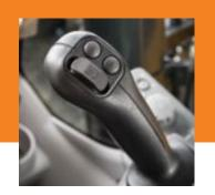
Ergonomically correct shortthrow pilot levers provide smooth, precise control with less effort. Pushbuttons in the right lever allow control of auxiliary hydraulic flow for attachments. Optional sliding switch provides proportional speed control, giving you full command from your fingertips.
