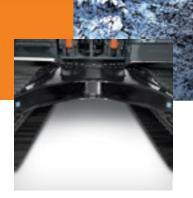
Thick-plate single-sheet mainframe, box-section track frames and industry exclusive double-seal swing bearing deliver rock-solid durability.
